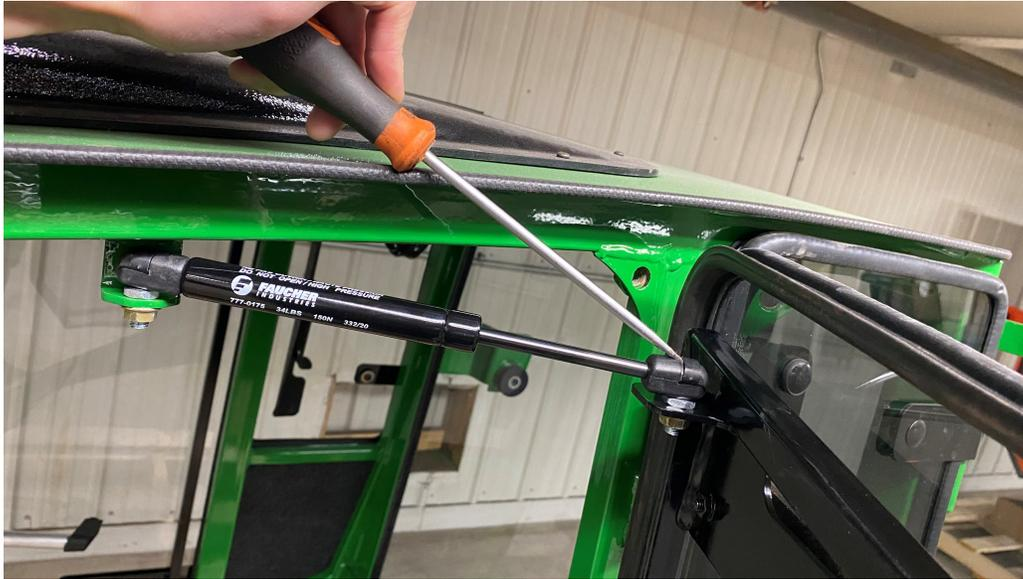
10. Take the provided cab lift bolts,  $\frac{1}{2}$ " x 4  $\frac{1}{2}$ " hex bolts, and install into lift weld nut that is located behind the tab at the top of the door opening.
