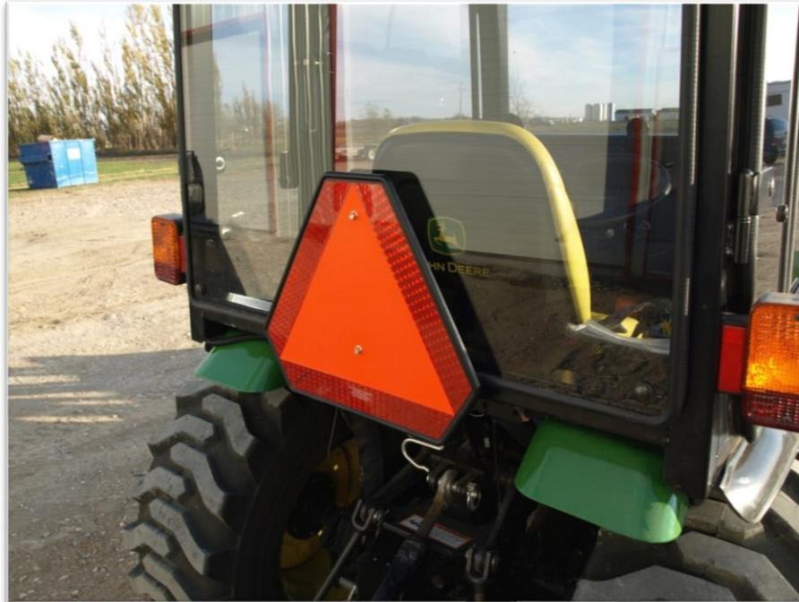
17. Take the left tractor flasher light and bolt onto the cab through the left C-post. Use the factory hardware. Route the wire harness through the centre large hole and down the post. Re-connect the wiring harness to the tractor harness. Repeat for the right flasher light.
