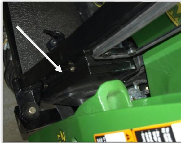
20. Take the left cab floor mat. Position it onto the left operator foot platform. Ensure that all pedals have adequate clearance to operate, notching if necessary. Using an aerosol spray glue, 3M High Strength 90 is recommended, and glue floormat into place.
