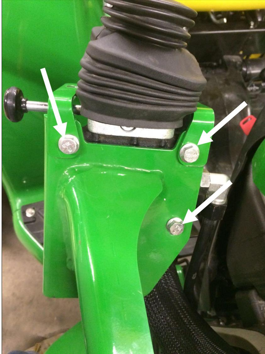
. Un-bolt the three fasteners that attach the loader valve bracket to the loader sub-frame shown on next page. Let the valve assembly hang as is.
