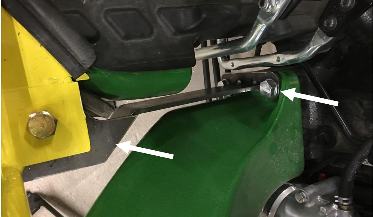
**NOTE:** For the right front bracket, the pedals are VERY tight to the bracket plate. It may be necessary to adjust the linkages to prevent interference to the bracket.
