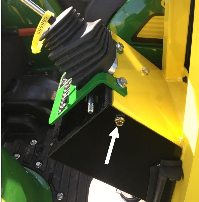
. Remove the SMV sign from the tractor. Fasten to the rear shield of the cab with the provided  $\frac{1}{4}$ " x  $\frac{1}{2}$ " flange bolts and nuts.
