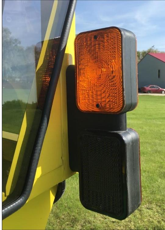
. Take the right flasher light removed earlier and route the harness through the large hole in the C-post. Fasten to the cab with the factory bolts and nuts.
