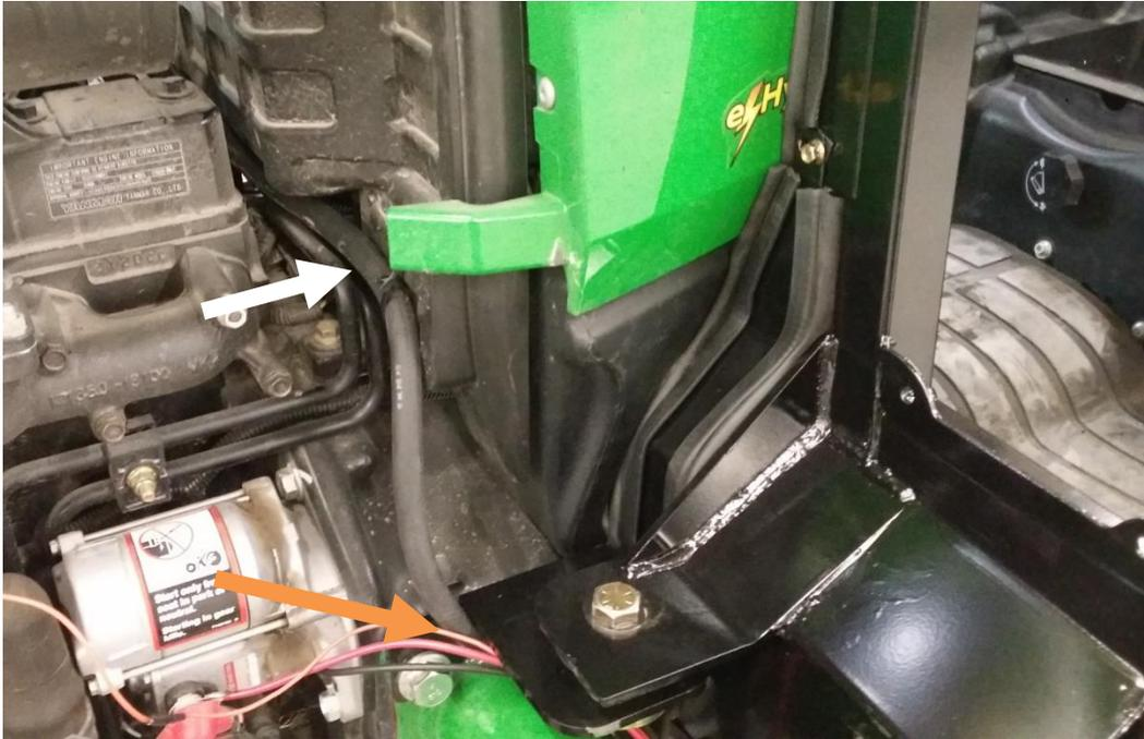
36. Take the hose coming out of the right A-post, and route into the engine bay, along the firewall, and up and over the air intake towards the open fitting on the water pump. Shorten hose if necessary, then connect to fitting. Use the provided HS-6 hose clamp to tighten hose.
