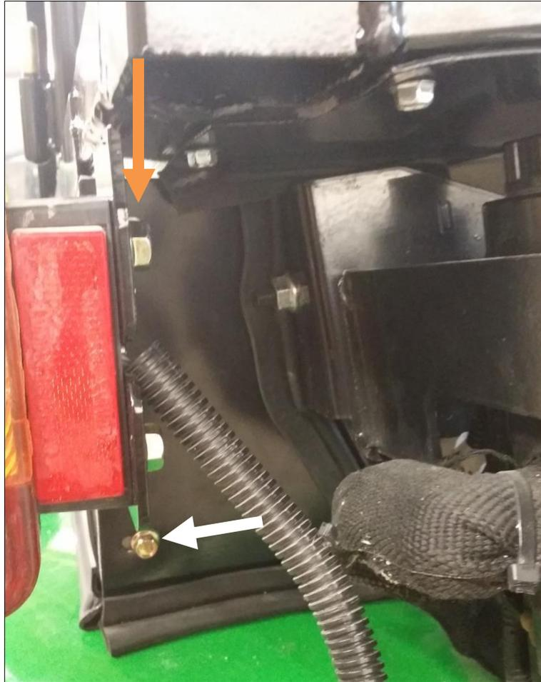
28. Take the right rear side fender shield and position against the 2-post ROPS, right side cab panel, and the rear shield. Ensure a good seal to 2-post ROPS, then fasten to cab with two of the provided 1/4" x 1/2" flange bolts. NOTE: This joint needs to be sealed with black silicone.
