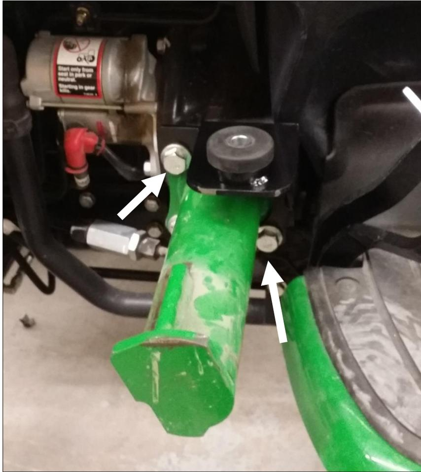
13. If equipped with loader, remove top two and bottom rear loader fasteners at the bell housing. Take the right front bracket and position into place, then use factory hardware to install bracket over load sub-frame. If no loader is present, use the provided spacers and the M16 x 40 bolts.
