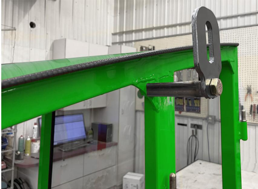
16. Attach a lift strap or chain to the lift brackets, and using a hoist or forklift, prepare to lift cab up off of the shipping pallet. Un-bolt rear shipping bracket from cab, and lift cab. Position the cab over the tractor.
