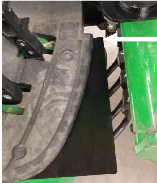
**NOTE: If tractor does not have a loader, washer spacers are required behind the front mounting brackets. Photos below have loader installed.**
