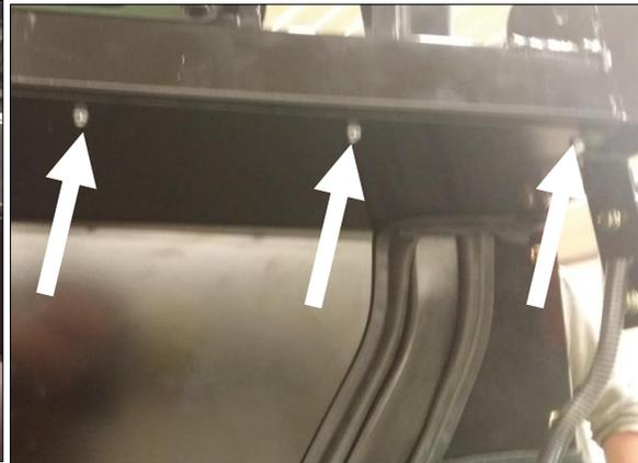
27. Take the left rear side fender shield and position against the 2-post ROPS, left side cab panel, and the rear shield. Ensure a good seal to 2-post ROPS, then fasten to cab with two of the provided 1/4" x 1/2" flange bolts. NOTE: This joint needs to be sealed with black silicone.
