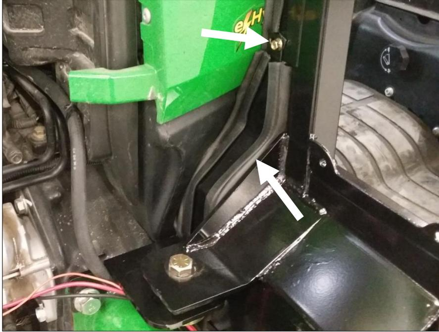
30. Take the right front under-hood shield and slide into position up against the cab and the tractor. Ensure good fit, then fasten into place with 1/4" x 1/2" flange bolts.
