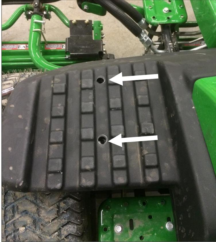
Un-bolt the bracket shown below to free up the back of the left side pod and the battery.
