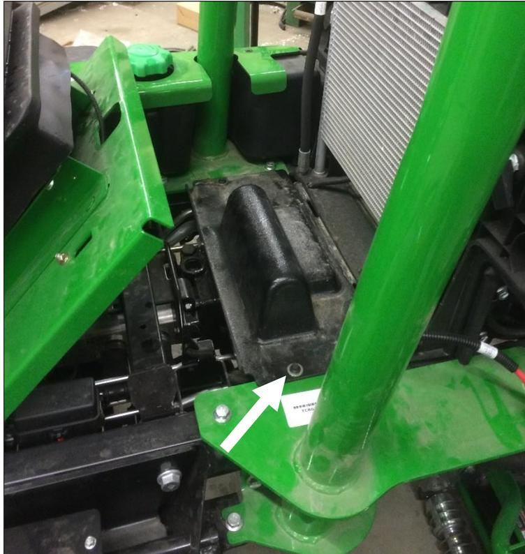
Un-fasten the green cover over the right side pod and remove from machine.
