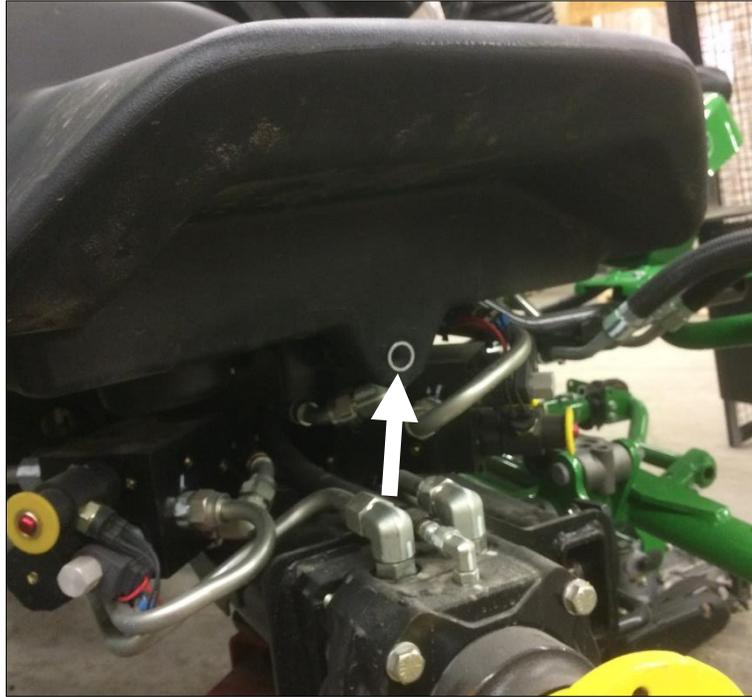
Support the fuel tank, and then slide outwards to gain access to the ROPS fasteners.
