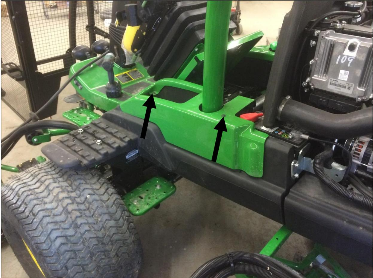
Remove the fasteners through the top of the black left side pod.
