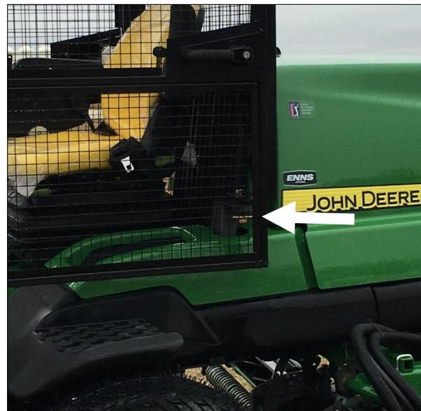
Get ALL fasteners started before applying ANY final torques. Tighten ROPS fasteners first, then tighten bracket fasteners.
