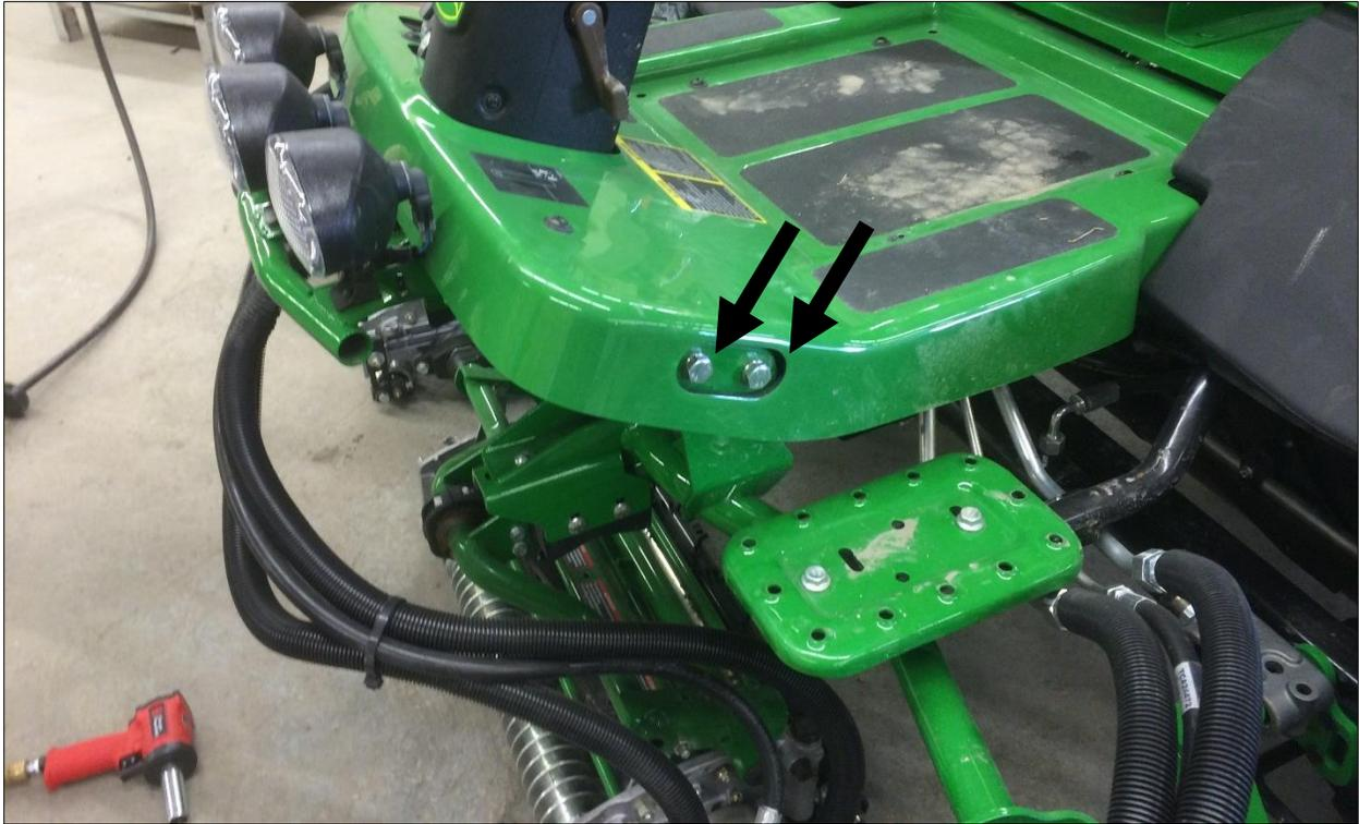
Take the left front bracket and squeeze in between the platform and steel plate inside of platform. Use factory hardware and bolt bracket into place. NOTE: steel sub-frame will want to fall down and out once fasteners are removed. (Right side shown below)
