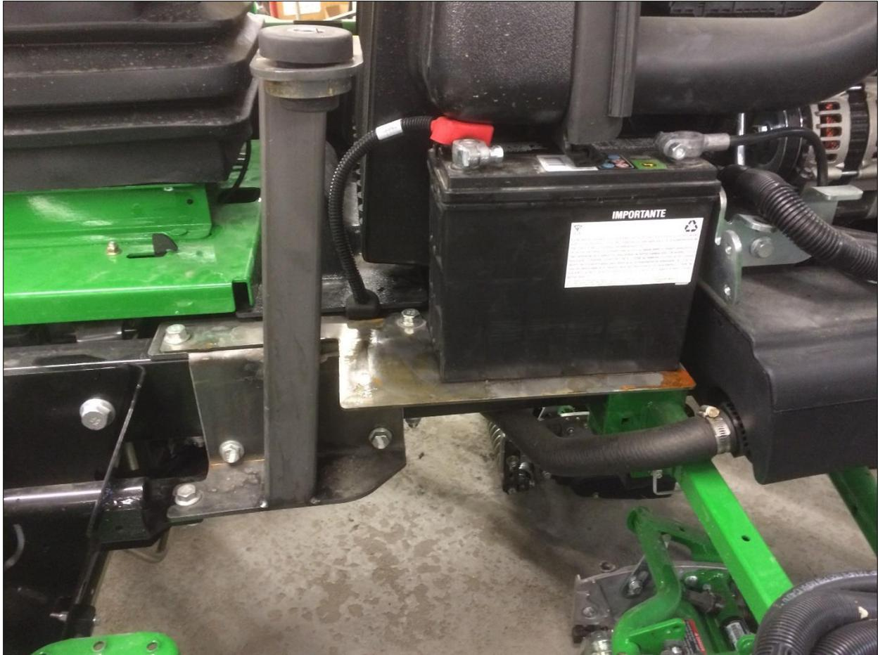
Take the right rear bracket and LOOSELY fasten into place with factory bolts.
