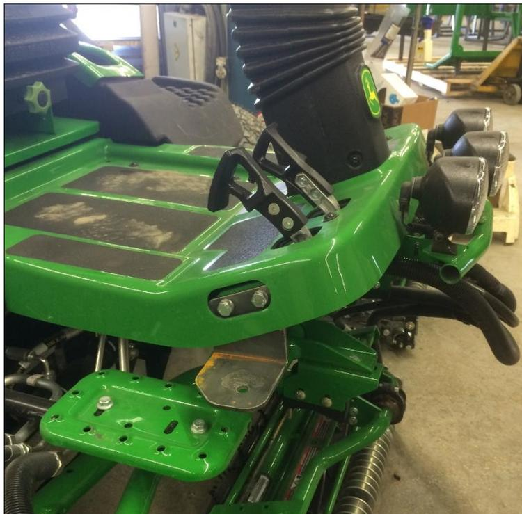
Remove holes from right side of platform and repeat procedure for installing the right front bracket.
