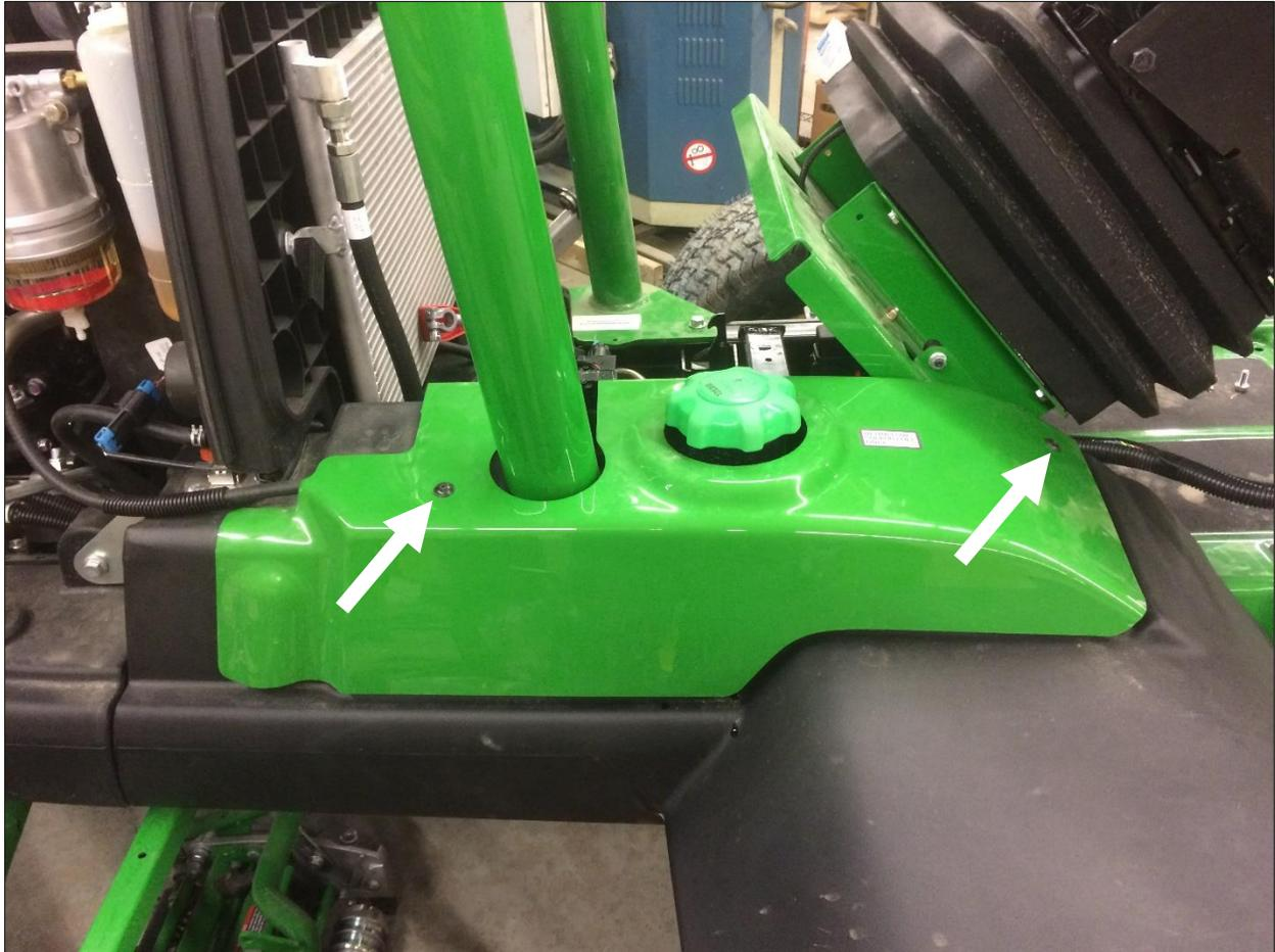
Slide the green side pod cover off of the fuel tank and off of the machine.
