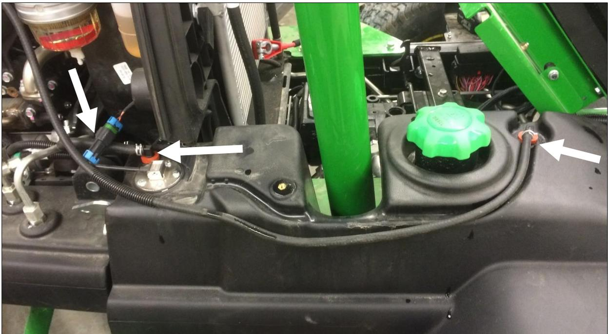
Remove the bolt shown here on the fuel tank.
