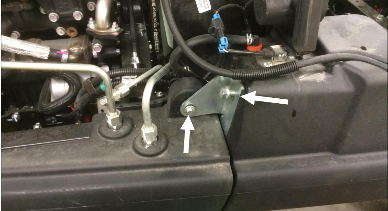
Disconnect the sensor and the fuel hose line at the front and back of the tank. This will later allow COMPLETE removal of the fuel tank from the mower chassis.
