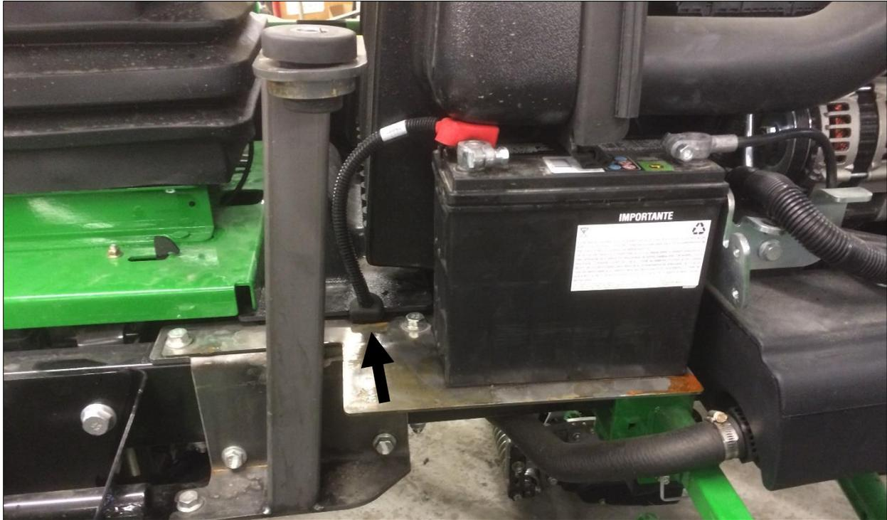
Push left tank back into place and re-install fasteners along with rear fastening bracket under hood.
