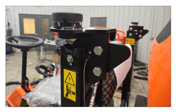
. Take the right rear bracket and position into place where the right side upper hoop of the 2-post structure was located. Use provided 1/2" x 1" hex bolts and loosely bolt the bracket into place.
