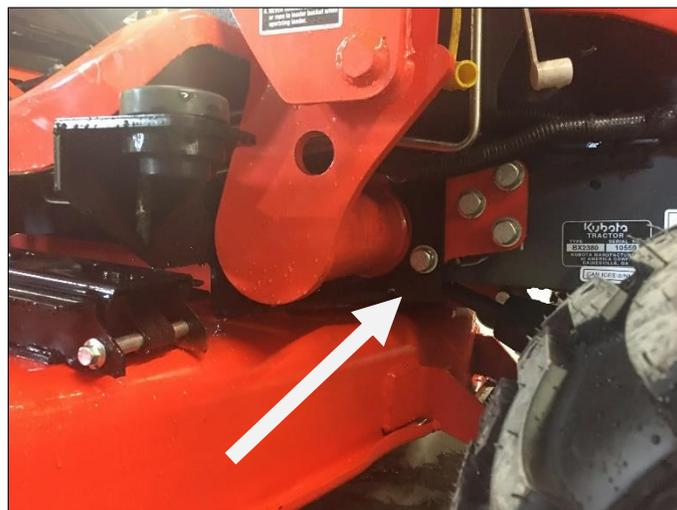
8. Take one of the rear brackets and slide it into the open socket where the 2-post ROPS was mounted on the left side. Use the factory hardware to fasten bracket to the tractor.
