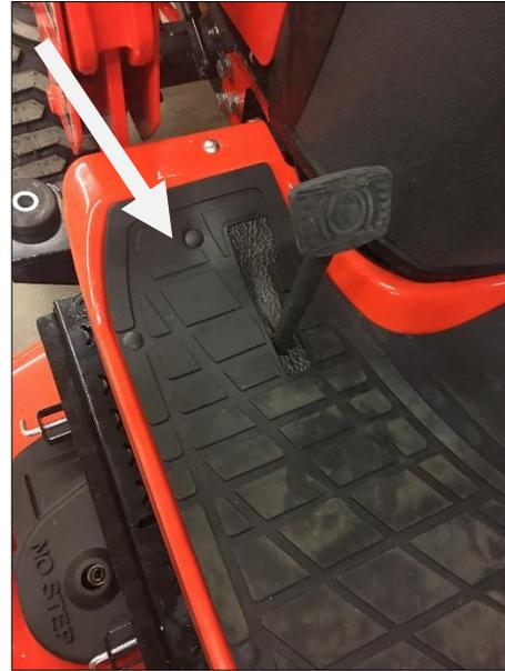
3. Re-install the left side of the platform floormat with the new fir tree fasteners provided.
