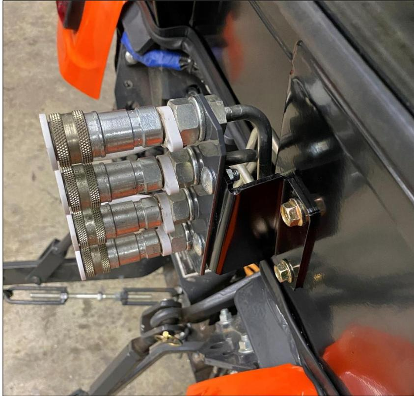
45. Position bracket against rear panel of cab and mark and drill two 5/16" holes using bracket as hole guide.
