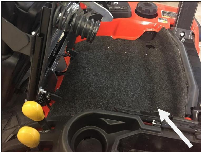
12. Remove the two cab doors by un-hooking the gas shock at the ball stud mounted to the door. To remove the gas shock on the left cab door, slide a flat screwdriver underneath the small clip on the end cap that must be pulled UP order to pop the shock off of the ball stud. **The**
