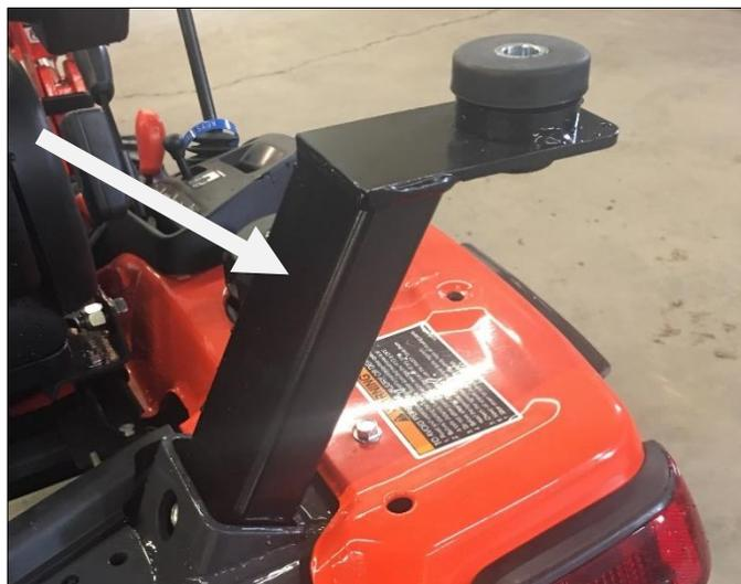
9a. Un-bolt and remove the left and right fender grab handles from the tractor.
