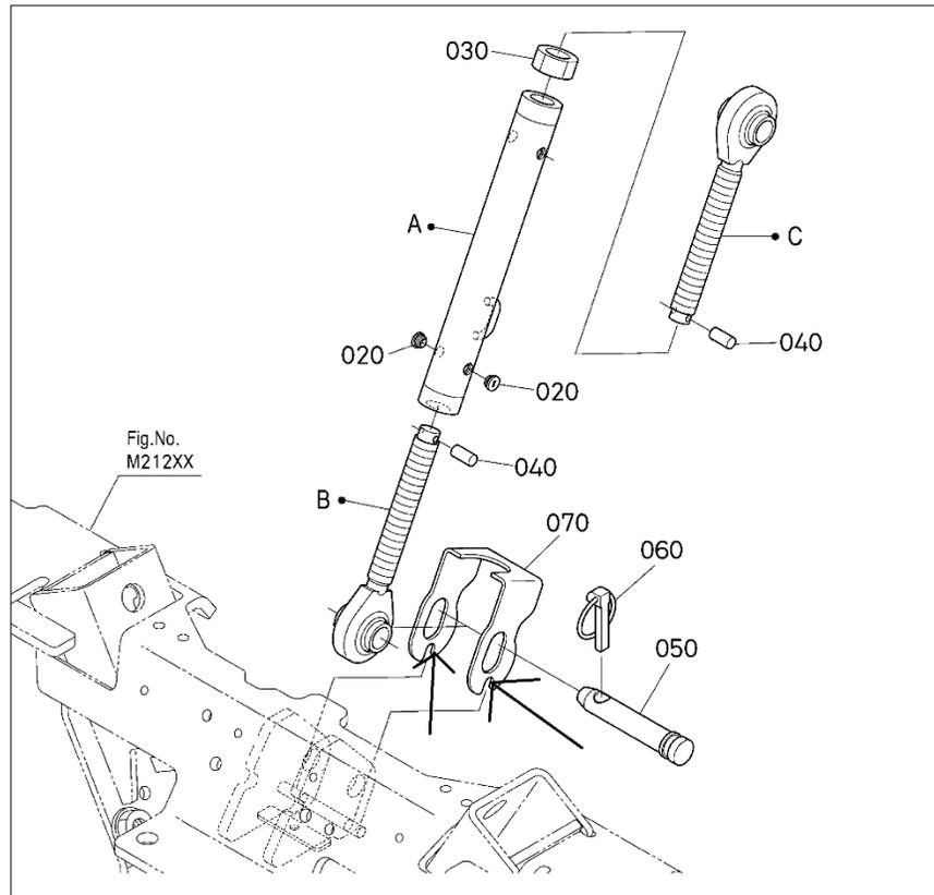
42. Note the arrows in the photo above, the bottom retainer notch needs to be widened by approximately 1/4" to allow the stopper bracket to be used when cab is installed.
