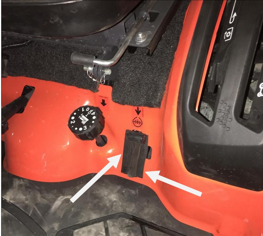
5. Disconnect rear flasher light harness and remove two-post ROPS from machine. Save fasteners to re-use later.
