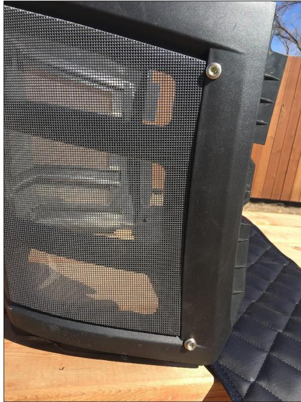
37. Wrap the winter front around the shroud, ensure it is tight, and mark the holes for the opposite side retainers.
