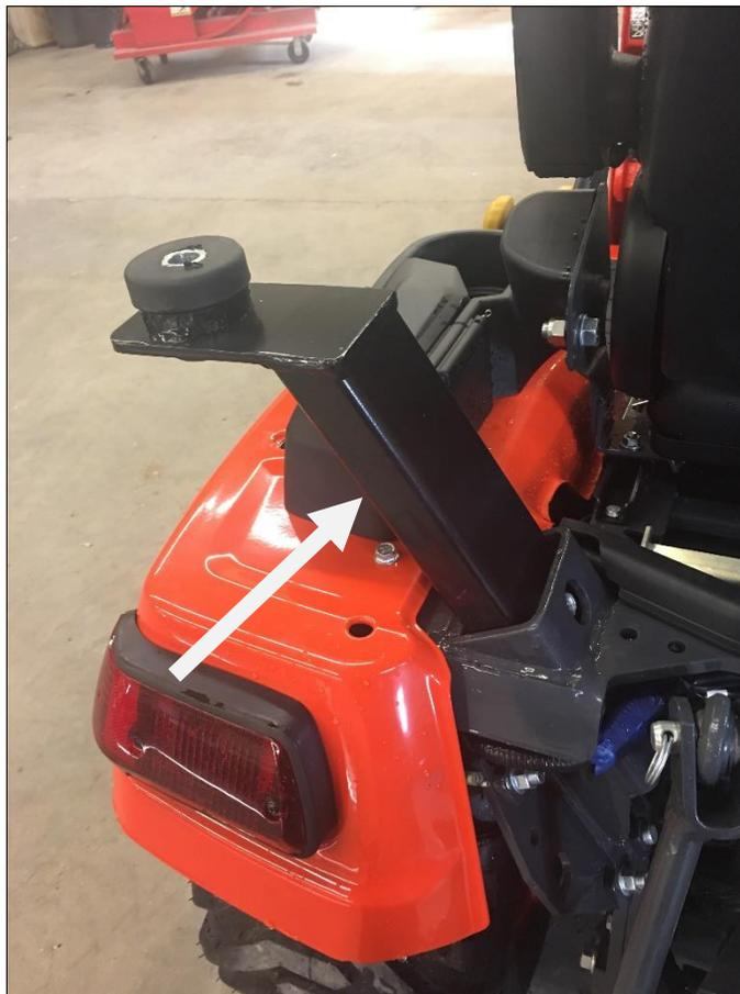
9. Take the remaining rear bracket and slide it into the open socket on the right side where the 2-post ROPS was mounted. Use the factory hardware to fasten bracket to the tractor.
