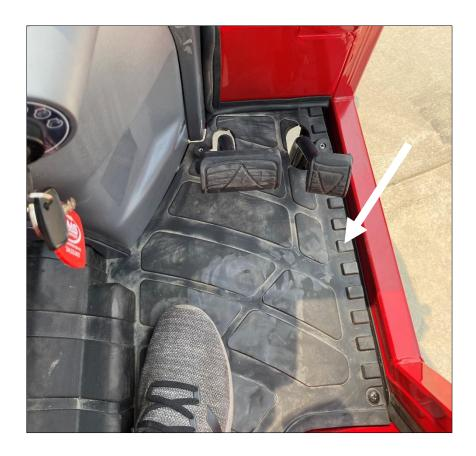
. To ensure a proper seal, use a black silicone around all the small open cracks between the cab weather stripping and the tractor.
