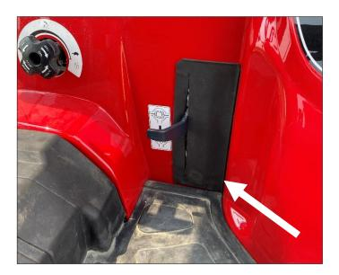
. Take the shorter adhesive neoprene piece and go to the right of the foot platform. Notch if necessary to allow control to slide through. Clean tractor surface for maximum adhesion, then pull off backing and install neoprene into place.
