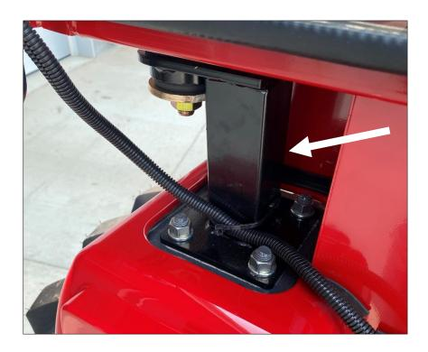
. Take the right rear bracket and position where the right side of the 2-post fastened to the chassis. Re-use factory hardware and loosely fasten into place.
