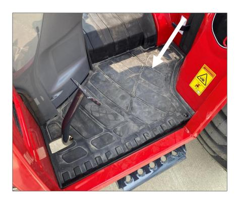
. Take the right platform floormat and position down onto right foot platform. Slide around pedals, ensure full range of motion, cutting floormat if necessary. Glue down onto foot platform with 3M High Strength 90. (Tektite floormat is not shown installed below)
